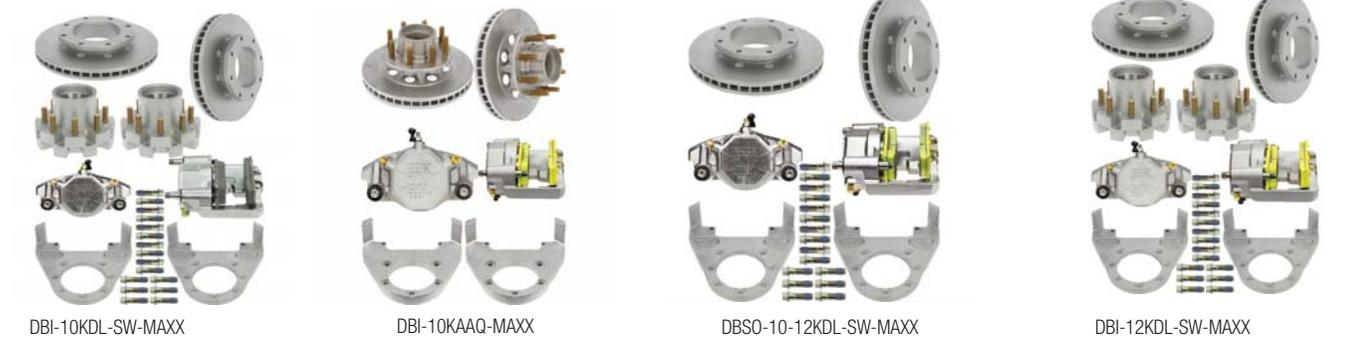
One (Axle) Set Of Integral 10,000 lb Maxx Disc Brakes For Dexter/Lippert Spindle
